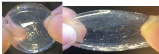
Figure 5. Photopolymerized PNIPAM hydrogel containing 10% clay (sample S2): (a) before and (b) after stretching. [Color figure can be viewed in the online issue, which is available at wileyonlinelibrary.com .]
